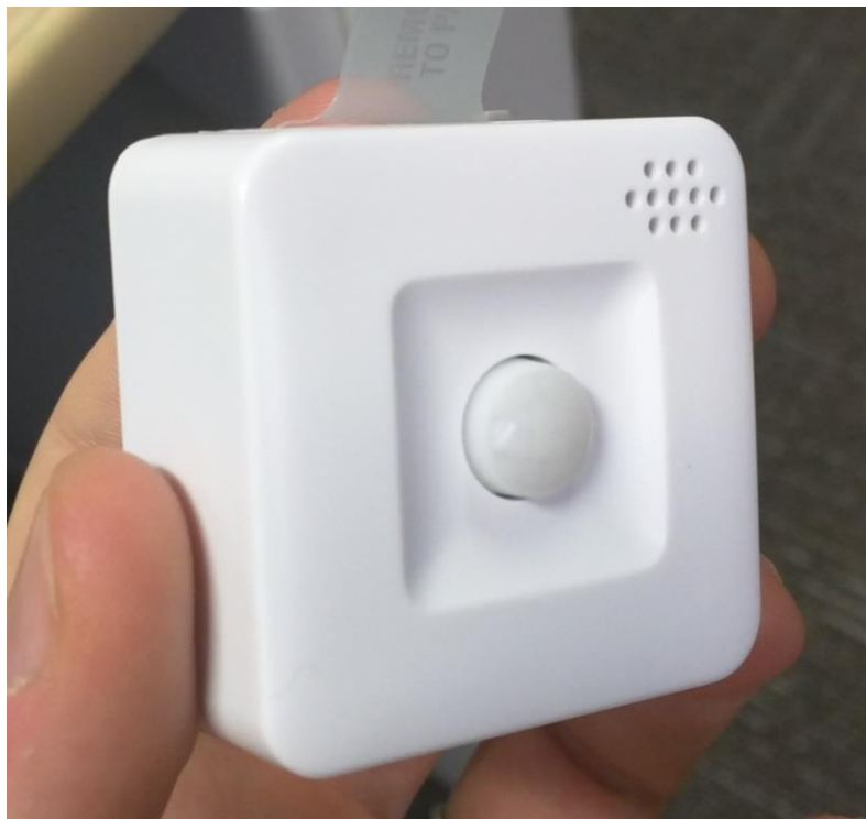
Figure 1 Battery powered Zigbee motion and temperature sensor selected for deployment
