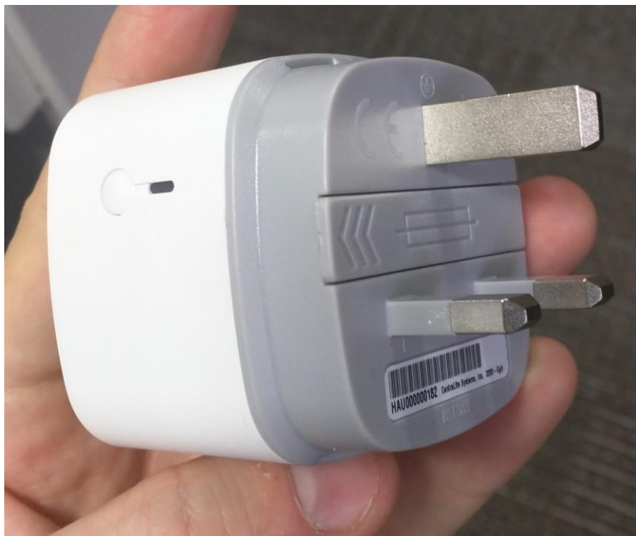
Figure 3 Rear view of smart energy metering outlet
